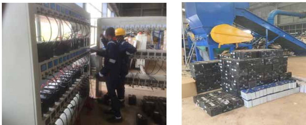
Figure 5: Staff at the lead-acid batteries testing and regeneration station (on the left) and regenerated batteries (on the right).
